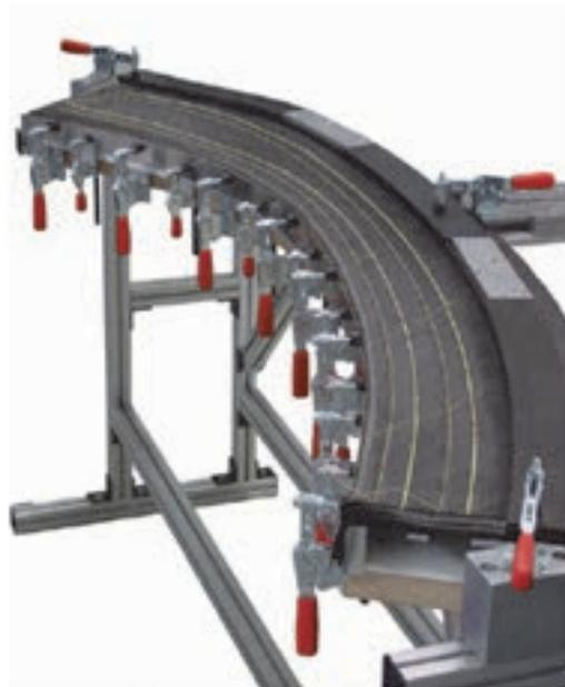
図 1.4.1 (3) - 3 Assembling of carbon fiber component from the aerospace
