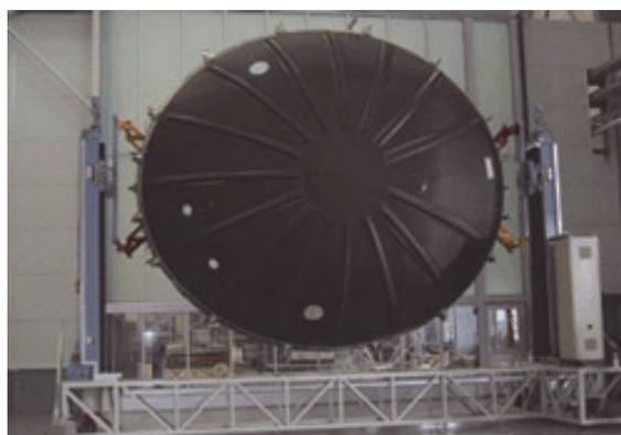
図 1.4.3 (2) - 1 A380 Aft Pressure Bulk Head
